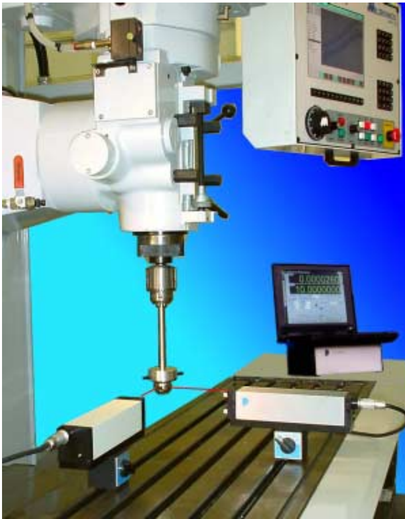
Fig.2 A photo of a typical setup for the measurement of spindle error motion
